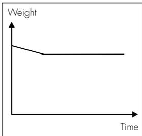
If the readout remains constant for a short time after a slight decrease in weight (as is the case with plastic granules), the automatic mode will not shut off.
