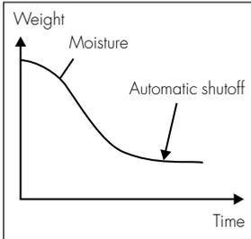
The fully automatic mode can be used when the weight loss during drying yields a curve that can be easily evaluated (such as the curve shown on the left).
