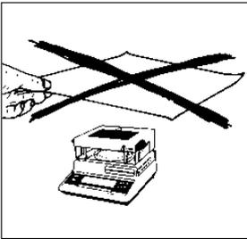
**When the moisture analyzer is being used, it gives off heat through the mesh on the hood. For this reason, the mesh must remain uncovered when the unit is in the standby mode and during operation.**
