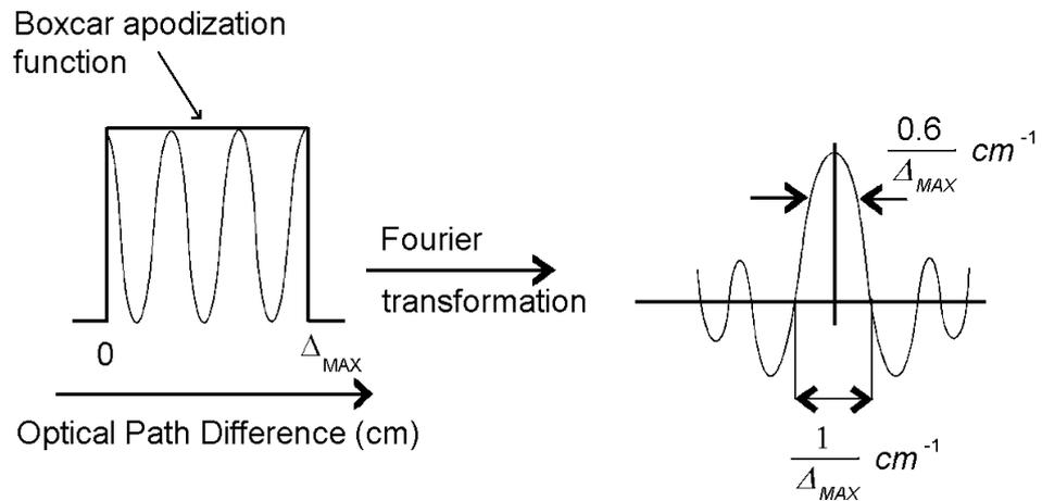
They can be reduced by multiplying the interferogram by a function which itself goes steadily to zero at the maximum path difference. This process is called apodization. The simplest function has a linear slope. Use of such triangular apodization reduces the sidelobes, which no longer become negative, but causes additional broadening.
