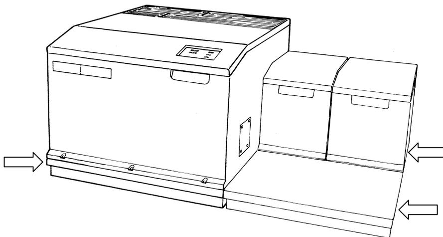
After the instrument has been moved to the position where it will be used, reverse the procedure you used above to raise or remove the shipping clamp so that the optical components can move freely.
