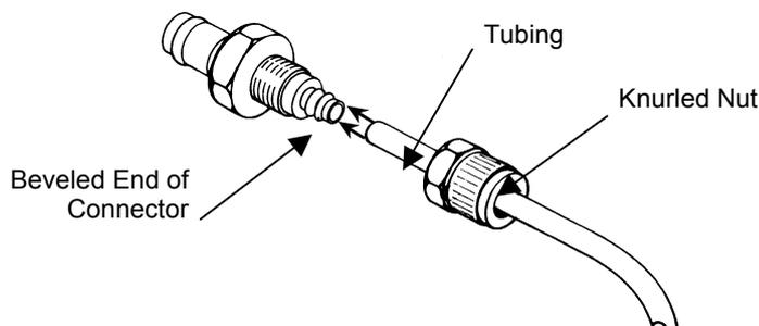
A tube fitted with one of these connectors can then be fitted to a purge inlet/outlet on the instrument. The purge inlet and outlet for the optical module is located at the back of the optical module. The purge inlets for the sample and detector areas are located on the side of the instrument.
