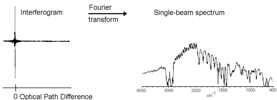
When no sample is present this gives a single beam spectrum, the overall shape of which is largely determined by the characteristics of the beamsplitter and source. Normally, interferometers operate by first recording this background and then ratioing the sample spectrum against it.
