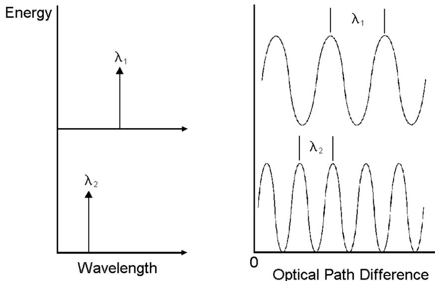
For a broad band source, the interference pattern is the sum of the cosine waves for all the wavelengths emitted. This interferogram consists of a strong signal at the point where the path difference is zero, falling away rapidly on either side. The customary spectrum, showing energy as a function of wavenumber, can be obtained from the interferogram by the mathematical process of Fourier Transformation.
