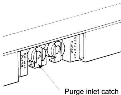
2. Pull the connector out of the purge inlet.
