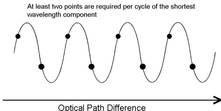
The sampling points for measuring the interferogram are derived from the laser signal. If one data point is recorded for each cycle of the laser signal, the data point separation is equal to the laser wavelength (in a vacuum) of 632.99 nm. The shortest wavelength that could be recognized in the spectrum would then be twice this laser wavelength, that is 1266.0 nm, corresponding to a wavenumber of  $7899\text{ cm}^{-1}$ .
