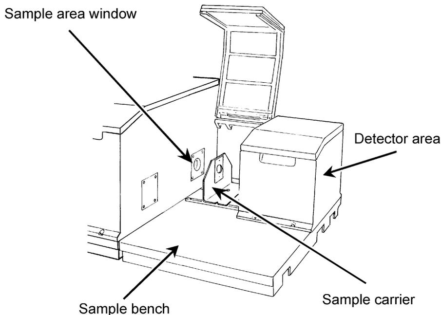
Sampling stations can be fitted to, and interchanged between, output beams as required.
