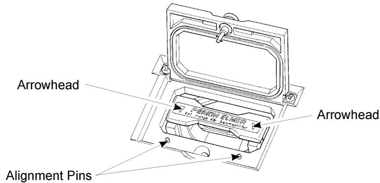
6. Insert the beamsplitter into the beamsplitter area, with the arrowheads pointing towards the alignment pins.
