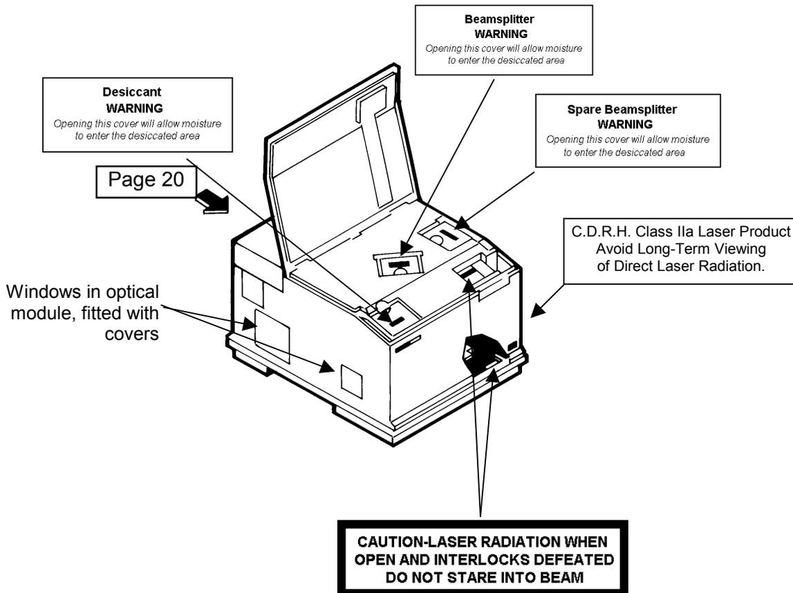
**NOTE:** *This label is for Service use only – the interlocks can only be defeated by a Service Engineer.*
