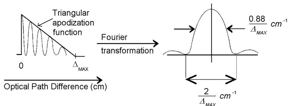
Various apodizing functions have been used, giving slightly different compromises between line broadening and reduction of sidelobes. Among these, the Norton-Beer functions ensure the smallest sidelobes for a given degree of broadening. The narrowest lines are obtained when no apodizing function is used, a situation sometimes called boxcar truncation.
